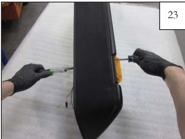
Secure the side marker light to the outer flare with Screw (SW1-0054), Nut (NU1-0018) and Washer (WA1-0003) using a #2 Phillips bit and a 11/32" socket with 6" extension. (2 places) NOTE: If you are having trouble putting the washer and nut on the screw, use needle nose pliers.
