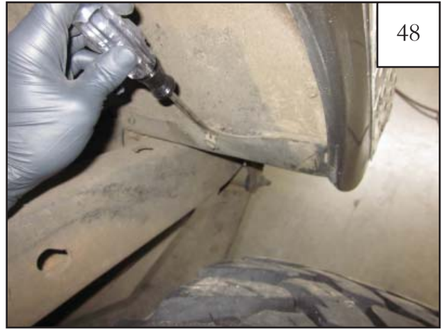
Using a pry bar or claw hammer, remove the christmas tree fasteners then remove/loosen the rear wheel well skirting. Save fasteners for reinstallation.
