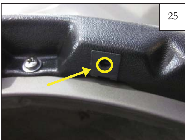
Before installing the outer flare, make sure that the Clips (CL1-0022) on the inner pieces are centered over the predrilled holes.
