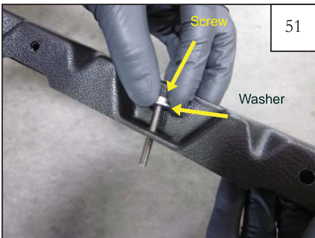
Put an Screw (SW1-0053) and Washer (WA1-0003) through the top holes of the inner pieces.
