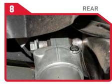
• The rear shock has a centered sleeve. • Torque the upper bolt to 56 ft-lb.
