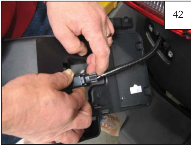
Reconnect light of license plate frame.
