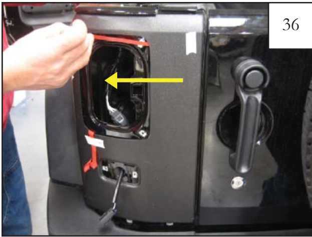
Pull tape liner 9 for the 1/4" tape to the left toward the driver side of the vehicle. NOTE: Refer to step 24 for tape liner tab numbering.
