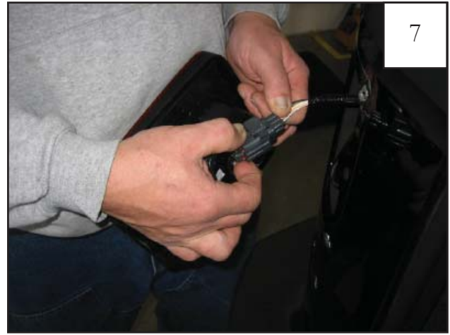
Disconnect the light by pressing down on the connector. Repeat steps 5-7 for passenger side tail light.
