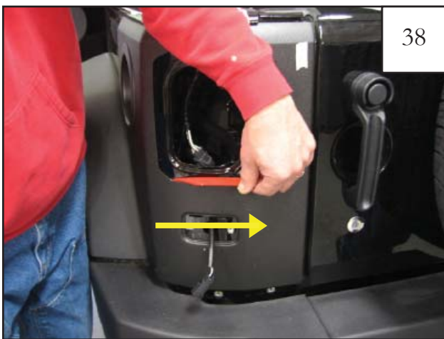
Pull tape liner 11 to the right toward the passenger side of the vehicle. NOTE: Refer to step 24 for tape liner tab numbering.
