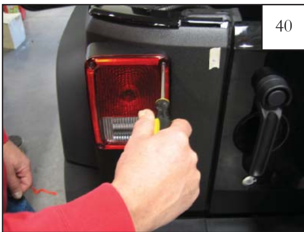
Using a #2 Phillips screwdriver, reinstall tail light.
