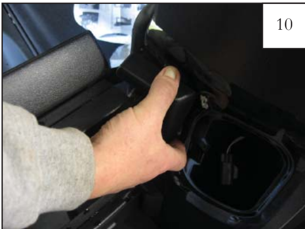
Slide covers off door hinges.
