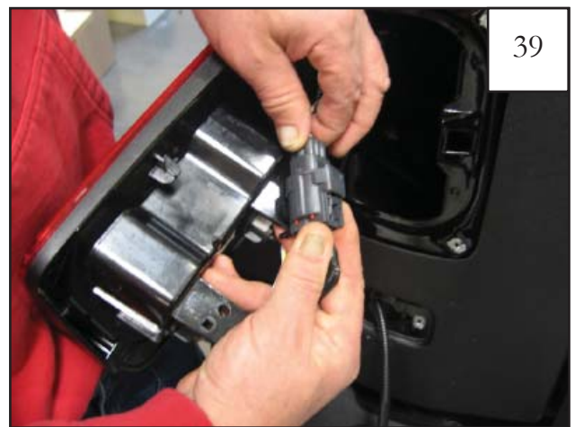
Reconnect light connector of tail light.
