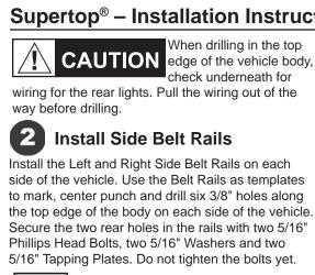
check underneath for wiring for the rear lights. Pull the wiring out of the
