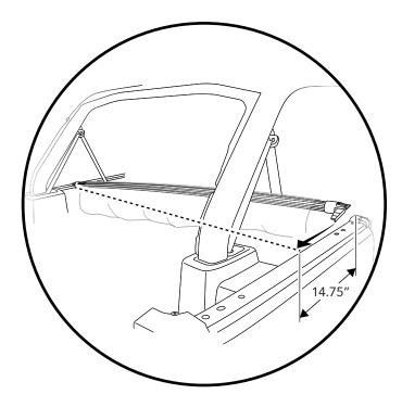
Now pivot the other end of the aluminum bow with attached end cap into place. Slide the opening of the end cap over the Jeep belt rail, and locate it the same distance - 14.75" - from the door opening trim cap on the same side.
