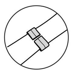
Place the lower strap between the two tabs on the lower side of the clip.
