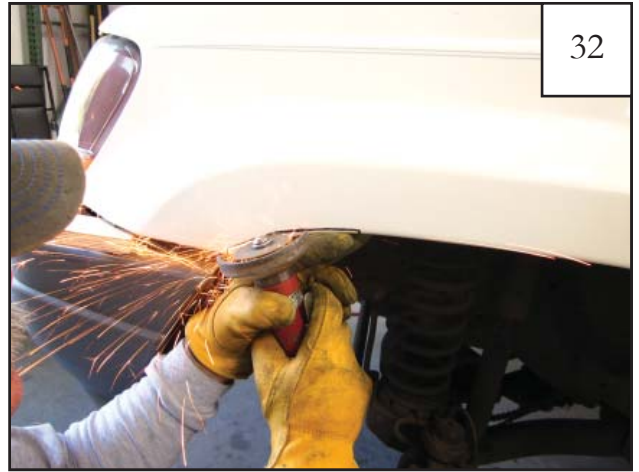
Starting at the front edge, cut out mark shown in Step 20. NOTE: Do not cut out the mounting point located at the front of the cut line.
