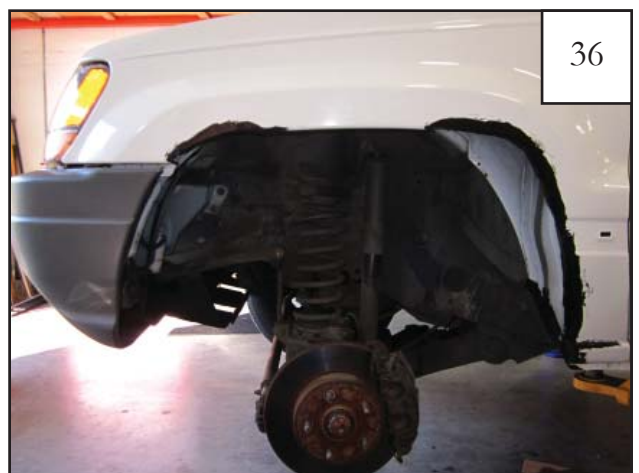
Completed cut-out with caulk applied.
