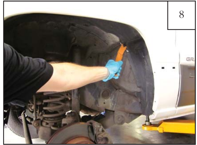
8 Using a pry tool or utility knife, remove factory fasteners from wheel well splash shield (9 places).
