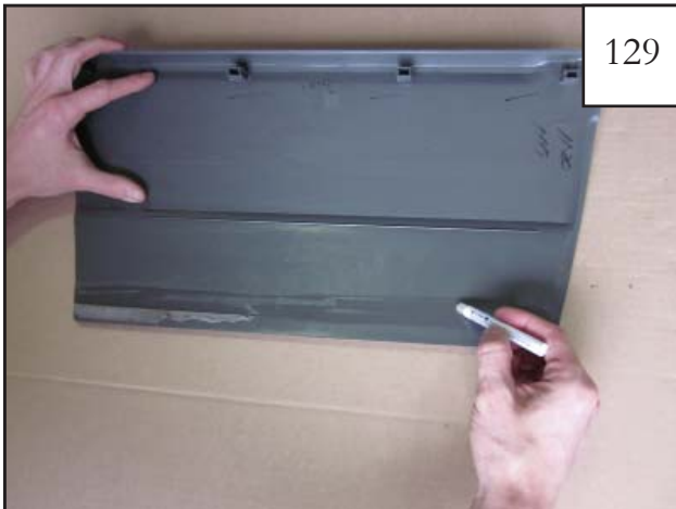
In preparation for applying new tape, apply primer using supplied primer applicator (AD1-0006) to plastic along bottom edge of side cladding.
