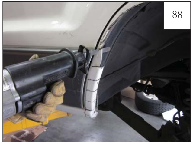
Using a cut off wheel, reciprocating saw or other suitable tool, remove tabs cut in previous step. Tip: Using a reciprocating saw works best for this cut. NOTE: DO NOT OVERCUT!
