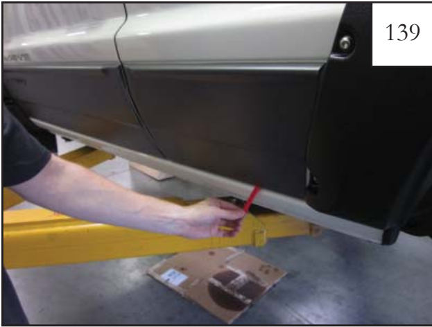
Remove tape liner and apply pressure to side cladding to adhere tape to sheet metal.
