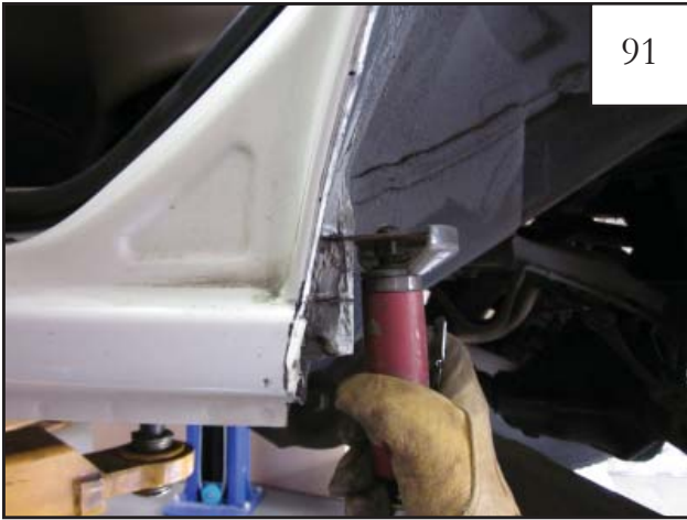
Using a cut off wheel or other suitable tool, cut along horizontal marks made in step 89.
