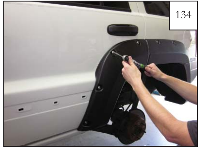
Hold flare in place on fender. Using the provided torx bit driver and ratchet with 3" extension, start each screw into drilled holes.
