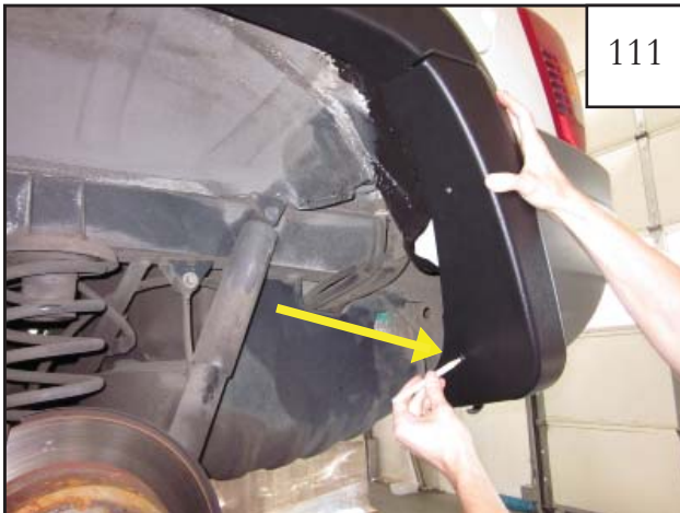
111 Hold flare and bumper piece in place so that the holes in the bumper piece barely overlap the cut bumper and mark the locations on the edge of the bumper. Use an awl if needed (2 locations).
