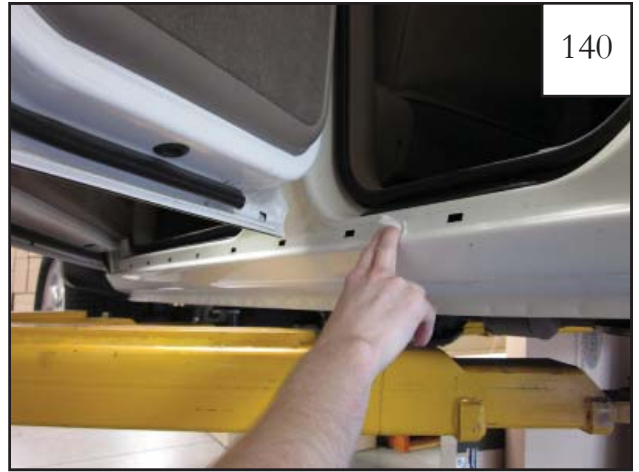
(NOTE: For models with previously removed Rocker Panels) Open front and rear doors. Remove dirt and debris from rocker area around holes in sheet metal. Then use supplied alcohol prep pad to clean and prep area prior to molding installation.
