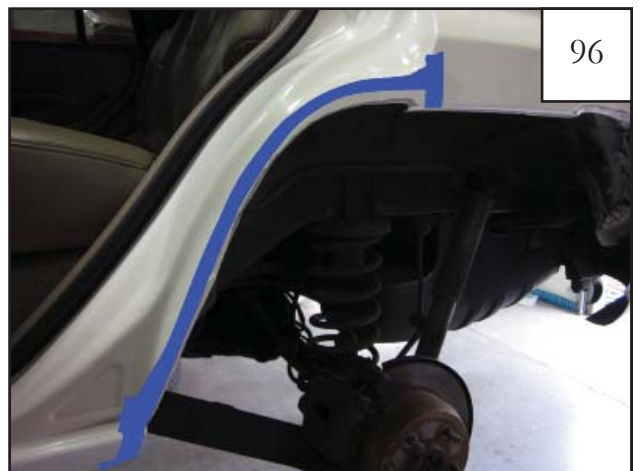
With door open, run masking tape along cut edges around door seam in preparation for sealing/caulking.
