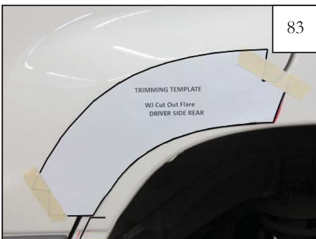
Using marks made in step 79 and 81 as a guide, set your supplied paper template on vehicle. Template should line up with both marks on either end. Outside curve of template should lay along style line on door. Template should be printed side up.
