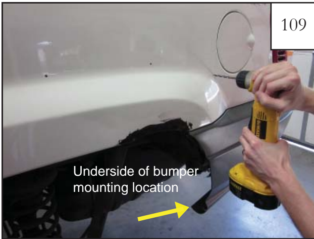
109 Drill holes in fender and bumper at marks with a 3/16" drill bit. Use 1/4" drill bit to drill mark on underside of bumper.
