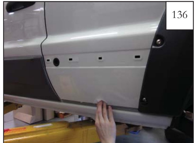
Prior to re-installation of the cladding, use a supplied alcohol prep pad to clean the sheet metal and any factory tape residue.
