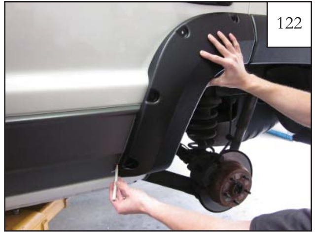
Close rear door. Hold door piece in place on door aligning it with rear main flare and trace outer edge of flare onto cladding
