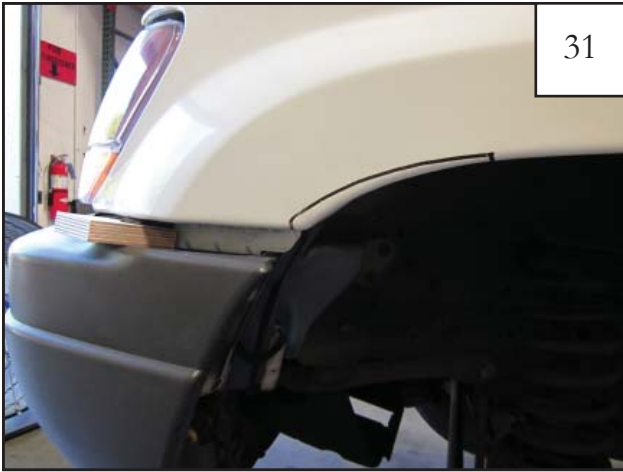
Use a small wood block to prop the bumper away from the fender in preparation for sheet metal trimming.
