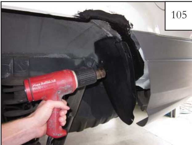
Using a heat gun, heat splash shield until pliable and use heavy work gloves to push and mold splash shield into place aligning with inner wheel well. Hold in place and allow to cool. Then fully install push retainers into splash shield.
