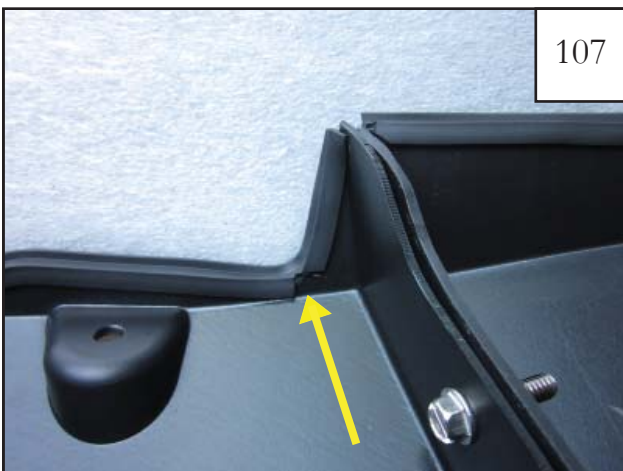
The Edge Trim (GP1-0005) on the sharp inside radius of bumper piece may need to be notched to fit correctly.
