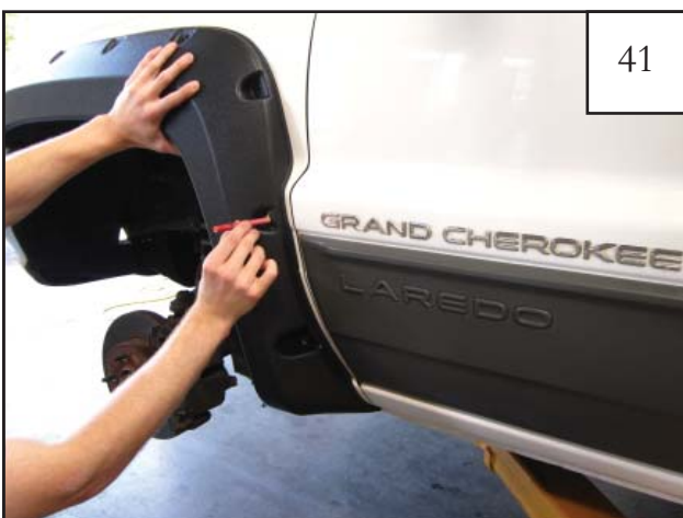
Hold flare in place on vehicle, mark hole locations on fender through holes drilled in pockets of flare.
