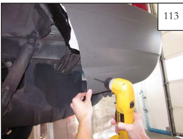
113 Using a 3/16" drill bit, drill the two holes marked in step 112.
