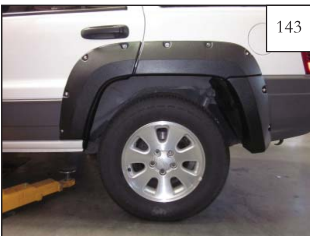
Completed rear flare installation.
