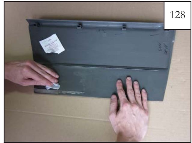
In preparation for applying new tape, use a supplied alcohol wipe (AD1-0010) to clean plastic and remove factory tape from side cladding.
