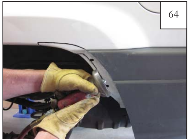
Using a cut off wheel or other suitable tool, cut along line marked in step 63 removing the inner flange.
