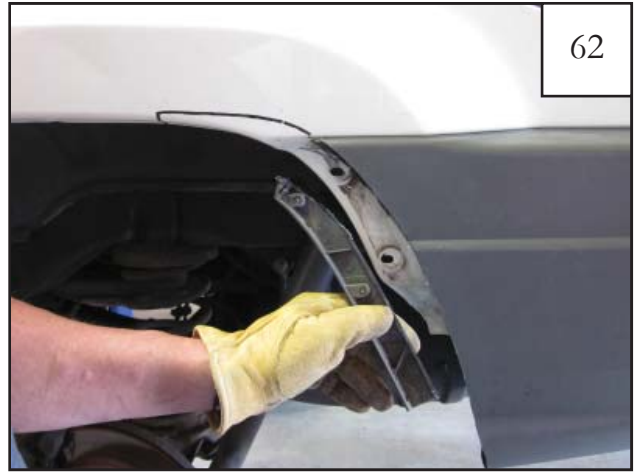
Remove trimmed bumper support bracket.
