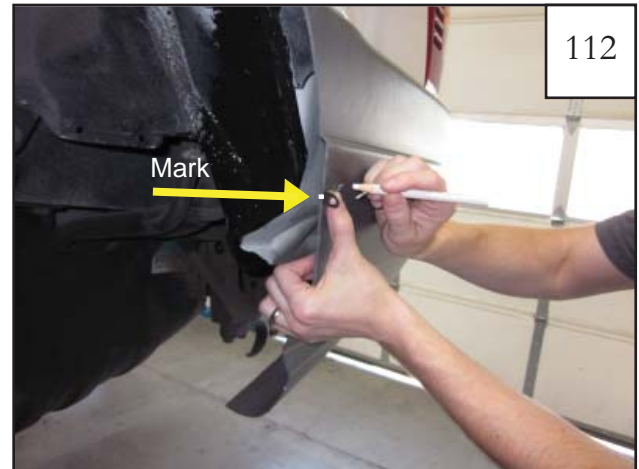
112 Hold mounting bracket (MB1-0003) in line with mark made in step 111 and make a mark through the hole location in the bracket. Repeat for second bracket.
