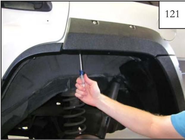
Secure flare to fender with panhead screw (SW1-0056) through holes drilled in step 120.
