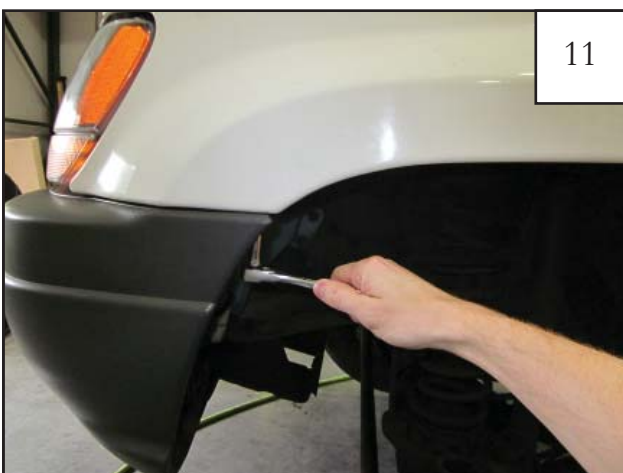
11 Using a 10mm socket and ratchet, remove factory screw from top of front bumper. Retain screw for re-installation.
