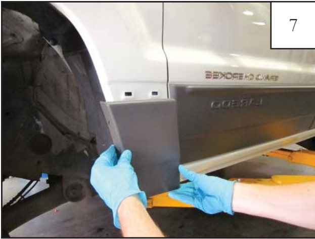
7 Pull firmly to remove upper factory fasteners in front side cladding piece from fender. Clean exposed sheet metal.
