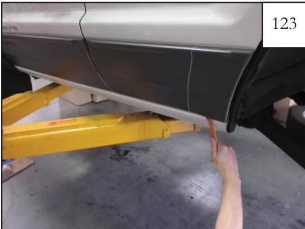
Using a pry tool, separate the factory side cladding from the sheet metal along the bottom taped edge.
