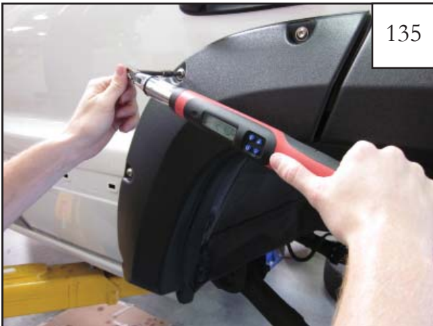
Once all screws have been started, snug screws to vehicle. Torque screws to 24 in•lb (2 ft•lb). DO NOT OVERTIGHTEN!
