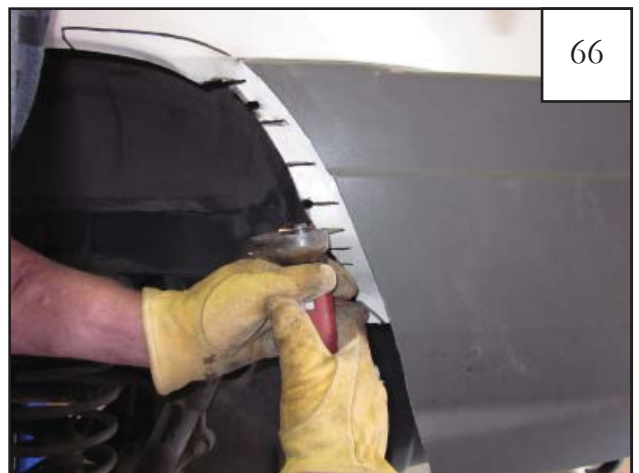
Using a cut off wheel or suitable tool, cut along marks made in previous step to create tabs.
