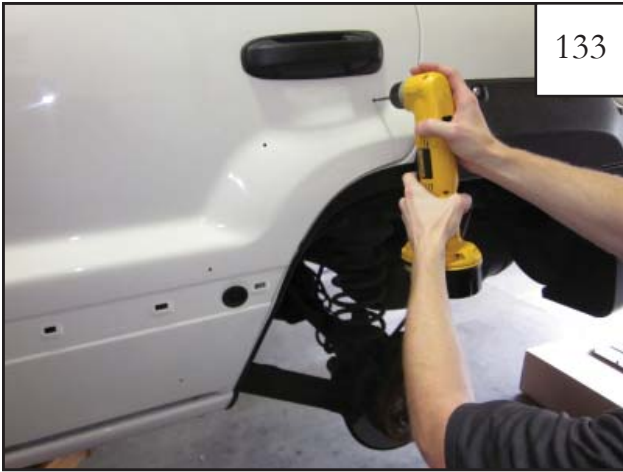
Using a 3/16" drill bit, drill holes marked in step 132.
