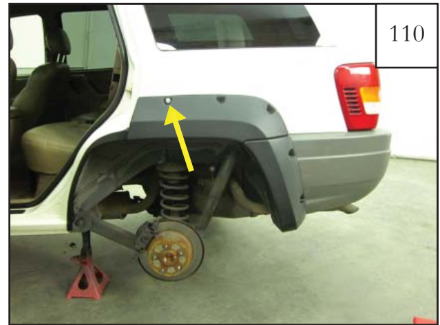
110 Install one screw (SW1-0045) in top front hole of flare to hold it in place while making marks in the next step.
