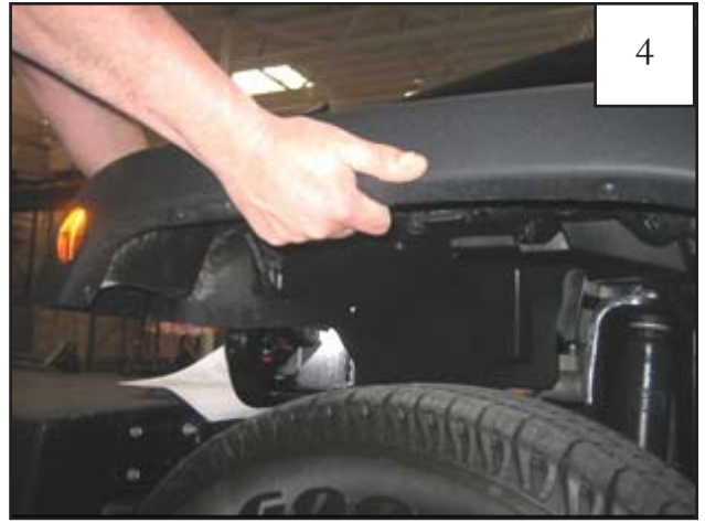
Starting at front of flare, pull firmly to release flare and splash shield from fender, working your way to the back. You will hear popping noises as clips release. It is okay. If clips break, they will be discarded.
