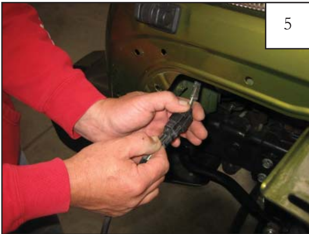
Once flare is free of fender, disconnect light connector. This will allow the flare to come away from fender completely. Save connector for reinstallation.
