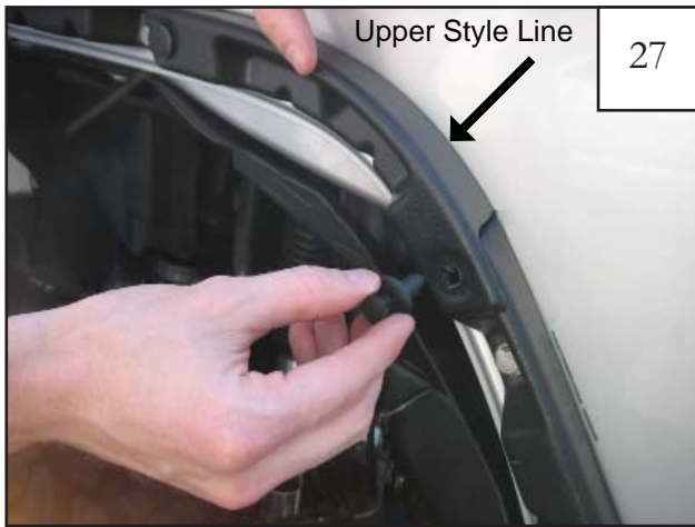
Step 2 While holding the inner piece in place, install a plastic push retainer through holes in both inner pieces. Inner piece should rest along upper style line of sheet metal radius and not below it: see step 22.
