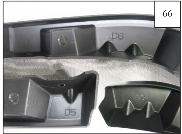
Locate the flat flare rear inner pieces. The driver side rear inner pieces are marked D5, D6 & D9. The passenger side rear inner pieces are marked P5, P6 & P9.
