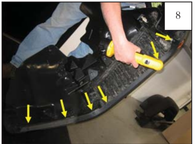
Use a drill with 5/16" bit to drill through six plastic rivets along edge of flare/splash shield. Discard flare. Save splash shield for reinstallation.
