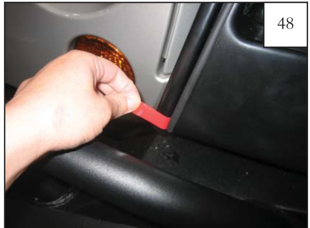
Pull tape liner from tape and press part to vehicle to secure adhesive backing. Tighten all Truss Head Screws first, then tighten all Torx Screws, moving from back to front.
