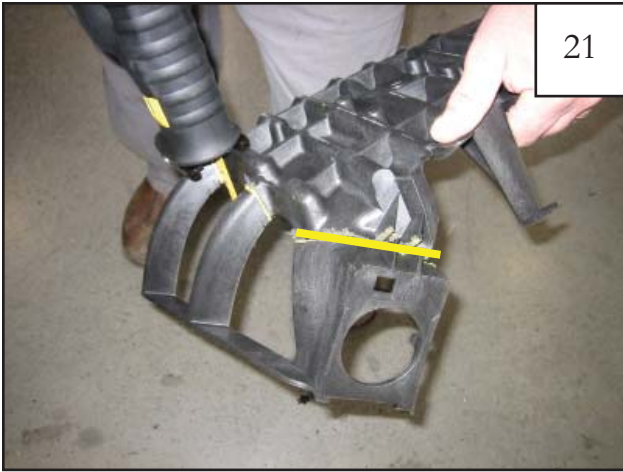
Using a hacksaw or saws all, carefully cut along lines made in Steps 19 and 20 to remove from portion of factory inner structure. Retain rearward piece.
