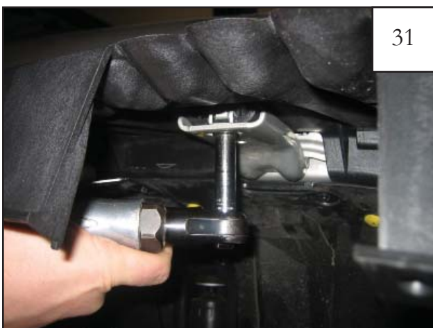
Tighten Bolt using a socket wrench with a 10mm socket.
