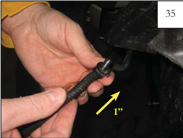
Slide the Christmas Tree Clip on light cord in towards vehicle body approximately 1"
