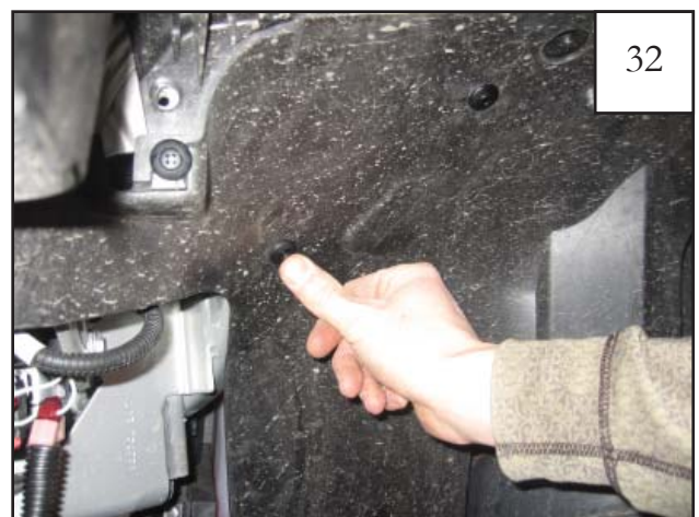
Install a supplied Plastic Phillips Head Tuf-lok in hole located towards the front of the splash shield.
