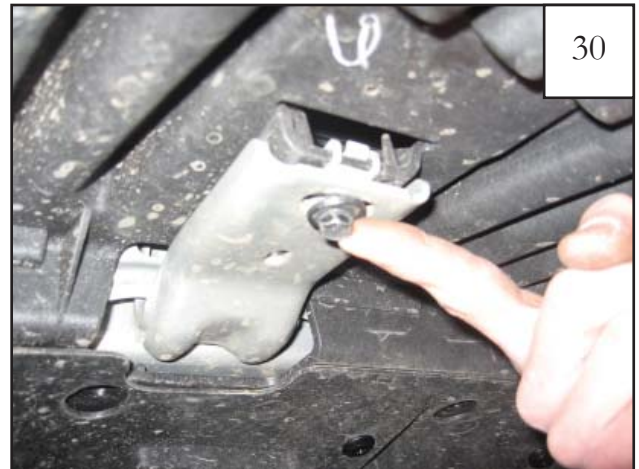
Start a factory bolt through inner structure and into brackets as shown. Note: It's easier to start bolts with your hands.
