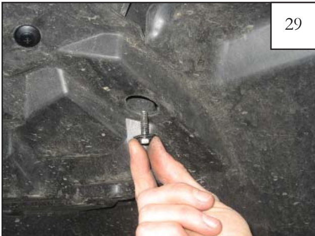
Reinstall the factory bolt through hole in splash shield as shown.
