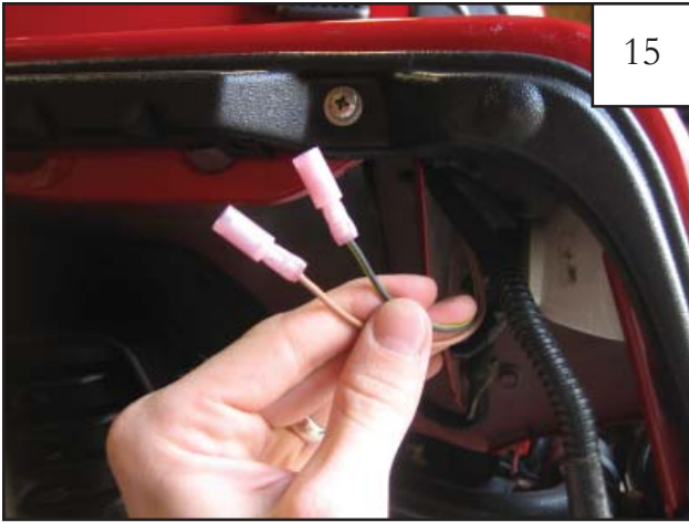
Install a Female Bullet Connector to the end of each factory side marker light wires and secure by pressing firmly with a wire crimp.
