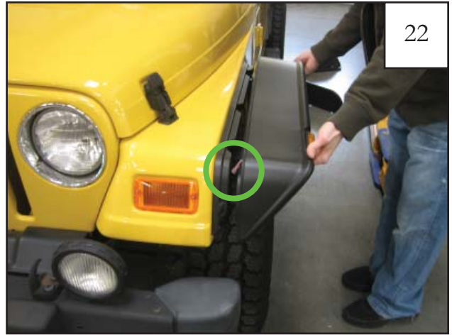
Place the outer flare over the inner pieces and push until snug against the sheet metal. Make sure that the side marker light wires are below the front inner piece.
