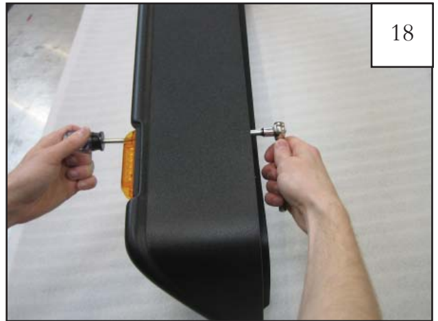
Secure the side marker light to the outer flare with 8-32 screw, 8-32 nut, and washer using a #2 Phillips bit and a 11/32" socket with 6" extension. (2 places) NOTE: If you are having trouble putting the washer and nut on the screw, use needle nose pliers.
