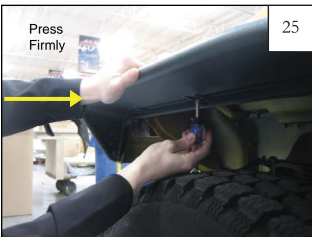
Tighten the #8 pan head screws by firmly pressing the flare toward the vehicle while tightening.
