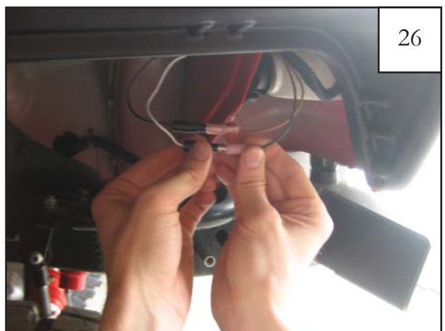
Connect the side marker light wires with the vehicle wires by attaching the male connectors to the female connectors. Test the connection by turning on the front turn signal. Switch connectors if necessary.
