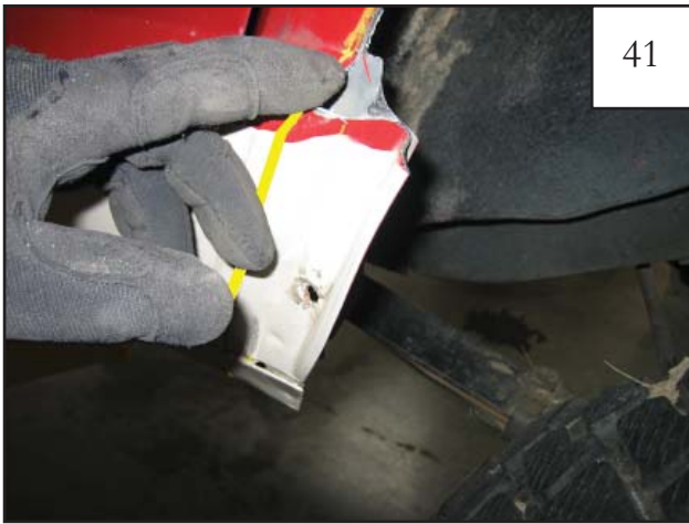
Along front fender well edge, cut through sheet metal down to the flare-out feature at the bottom.
