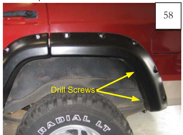
Optional: There are extra drill screws (SW1-0015) supplied in the kit. If desired, further secure the rear of the rear flare using drill screws. Place drill screw on part and drill into sheet metal.
