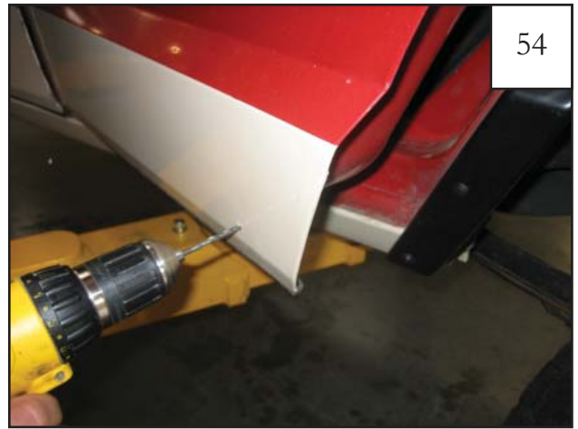
Open Door. Drill marks with a 3/16" bit.
