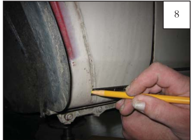
Starting at the edge of the door seam, measure in (towards fender well opening) 5-1/4" and make a mark.
