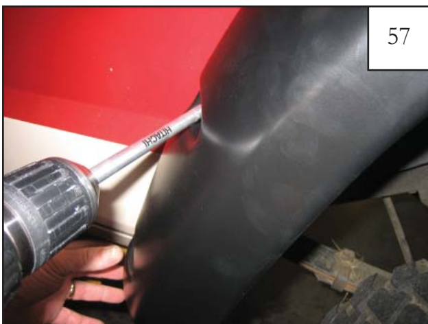
Start each screw with a T45 Torx bit in each pocket but do not tighten until all screws have been started. Over-tightening screws may cause them to strip! Use a Torque setting of 24 inch/ounces.
