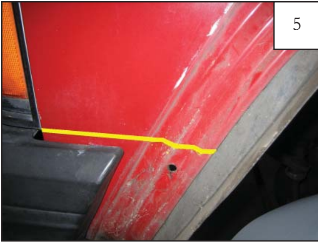
Using a grease pencil, make a horizontal line horizontally from the bottom of the headlight bezel to the inside of the fender well opening.
