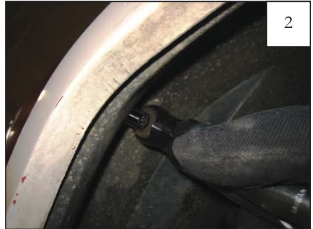
Using a 10mm socket, remove the factory fastener located inside the top front of the fender well.
