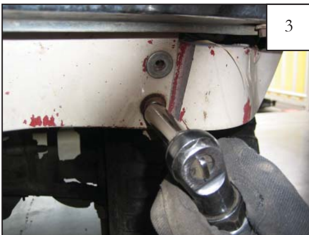
Using a 10mm socket, remove two factory fasteners underneath bumper on either side. Remove fascia piece
