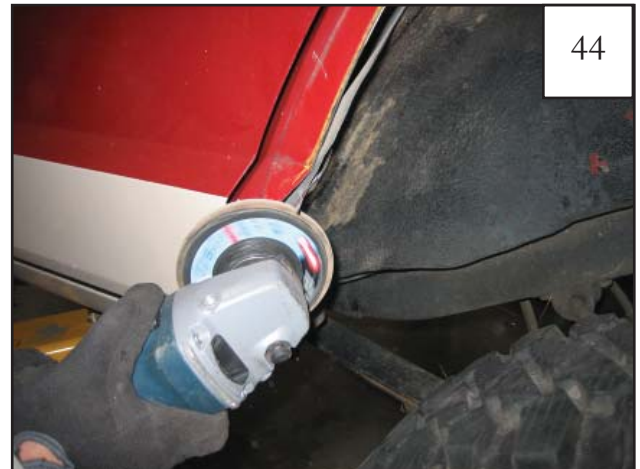
Grind back excess metal as needed. Trim the inner wheel well to match the contours of the sheet metal.
