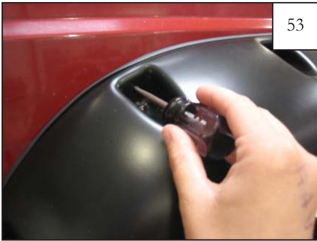
Using the holes in the part as a guide, mark hole locations on fender (4 places).
