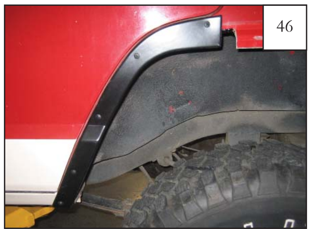
Open door. Install cover piece over "dog leg" using five supplied drill screws (SW1-0015). Place drill screw in indent in part and drill into sheet metal. NOTE: Some trimming may be required.
