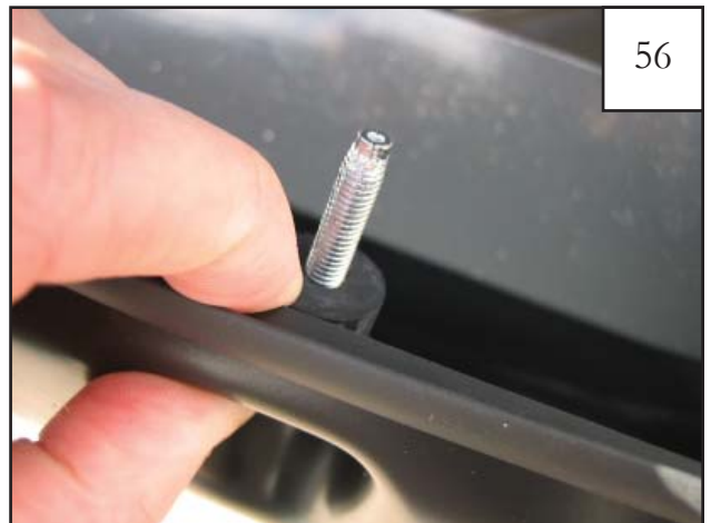
Place a 3/8" thick rubber spacer (SP1-0009) on each screw from the backside of the pocket. Threads must protrude through spacer for proper attachment of flare. All spacers must be installed prior to installation on fender.
