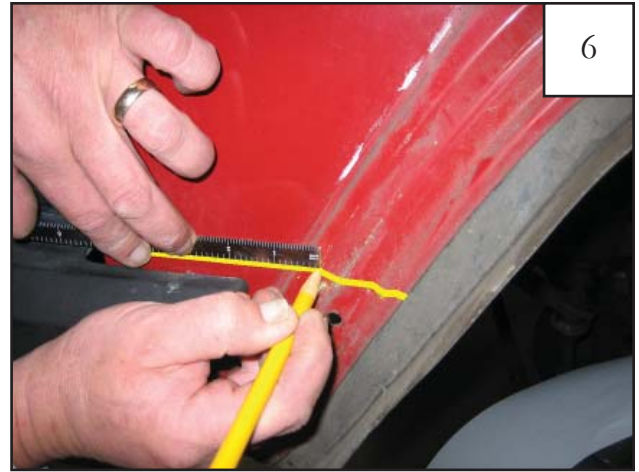
Starting at the bottom of the headlight bezel, measure in 5" and mark a line on the fender
