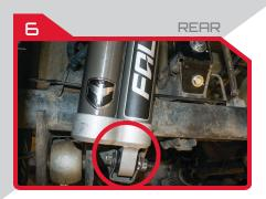
Install the shock's lower euelet into shock bracket.
