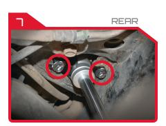
Torque upper bar pin bolts to 25
