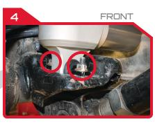
Install and torque lower bar pin bolts to 20 ft-lb.
