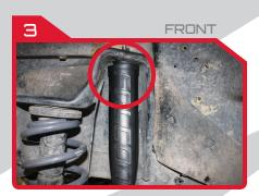
Install shock with roost guard facing outward.
