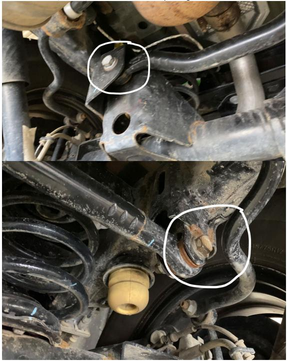
b. Note – you will need to slightly lift the passenger side rear to gain access to the bolt to remove.
