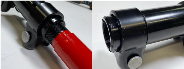
h. Once you have measured the correct length and assembled the track bar, this is the correct installation orientation:
