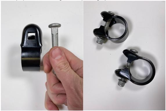
e. Slide the clamps onto the adjuster tube (preferably with the clamps nut facing the same direction), and then snug the nut up so that it still rotates but does not slide off using your 15mm socket or wrench
