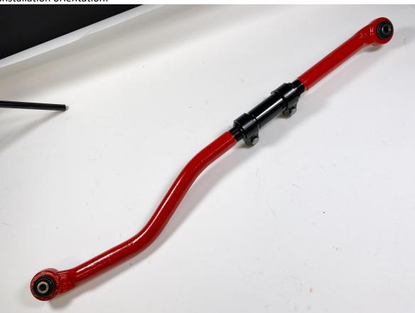
4. With the clamps still loose, it is time to install our track bar into the vehicle. Start by putting the passenger side end in and reuse the original 21mm fastener and nut – spin the nut on to hold in place but do not tighten yet.
