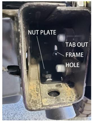
Remove Trailer Hitch Tab Plate
