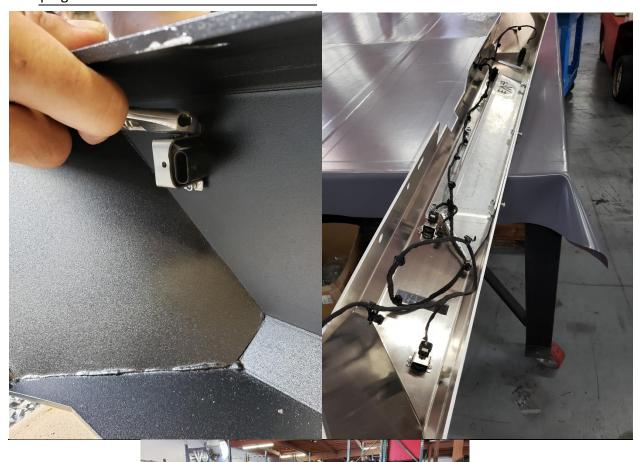
Careful when installing sensor hardware. Use a well fitted wrench and lightly tighten.
