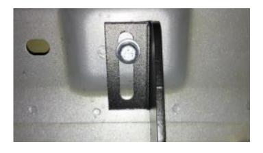
5. Attach the the Rocker Guard to the front of the pinch weld using the included M8 bolts and nuts.
