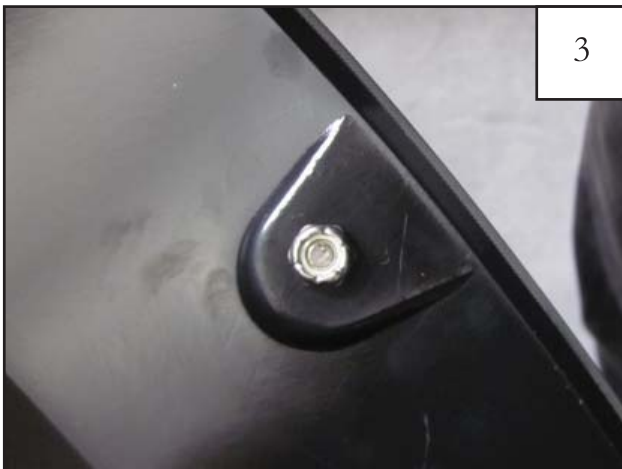
Place a Nut (NU1-0019) over the end of each Bolt and tighten, using a 1/2" wrench for the Nut and the supplied Torx Bit (SW1-0052) for the Bolt. Repeat for remaining pockets.
