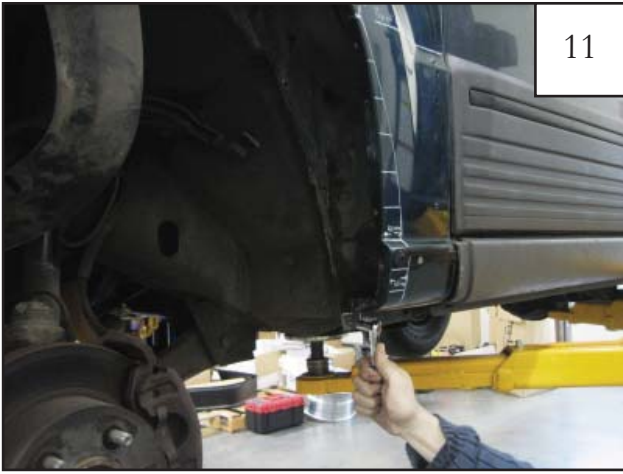
Remove and save factory bolt from bottom rear of front wheel well.
