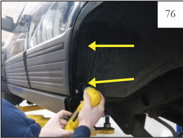
76 Remove part and drill marked locations with 3/32" drill bit.
