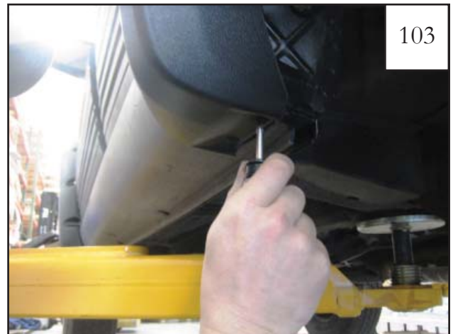
Fasten bottom of rocker panel piece with #8 pan head screws in holes drilled. A drill with a #2 Phillips driver works well.
