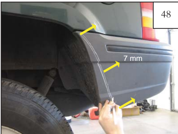
Trace a second line 7 mm offset from previous line toward rear of vehicle.
