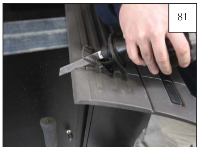
81 Using a reciprocating saw, cut the body side molding along line drawn in step 78.
