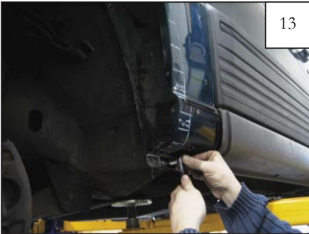
Install factory bolt saved during step 11 through the hole drilled in step 12.
