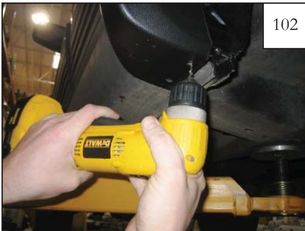
Drill 3/32" holes through holes in bottom of rocker panel piece through factory plastic and sheet metal.
