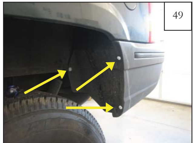
Remove three plastic factory fasteners with a Phillips screw driver and remove the liner. Fastener heads may need to be cut off with a utility knife. Fasteners are white in picture for visibility.
