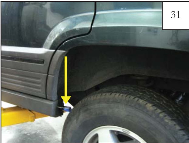
Using a stubby Phillips screwdriver, remove screw from rocker panel at forward side of rear wheel well.
