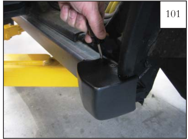
Fasten top of rocker panel piece to door sill with #8 pan head screws. Close door and verify alignment with door piece. Loosen screws and adjust if necessary.
