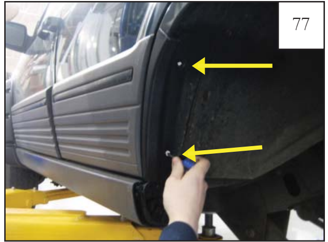
77 Place cover piece back on "dog leg" and fasten with two #8 pan head screws. Screws are white in picture for visibility.
