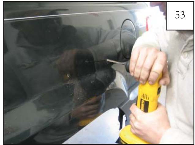
Drill holes in fender and bumper at marks with a 3/16" drill bit.
