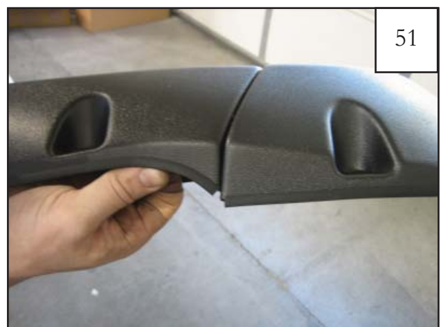
For edge trim application on rear main flare and bumper piece, follow steps as listed at the beginning of this instruction set. To apply edge trim around area where the two pieces connect, refer to this image.
